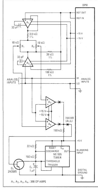
**Limit checker.** Potentiometers define upper and lower threshold for permissible range of analog signal. When input is above or below the threshold range, the timer, connected as an astable multivibrator, begins to flash either the entire display or its polarity sign.
